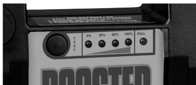
Test Button, Charging, Power Levels and Charge Complete LEDs
